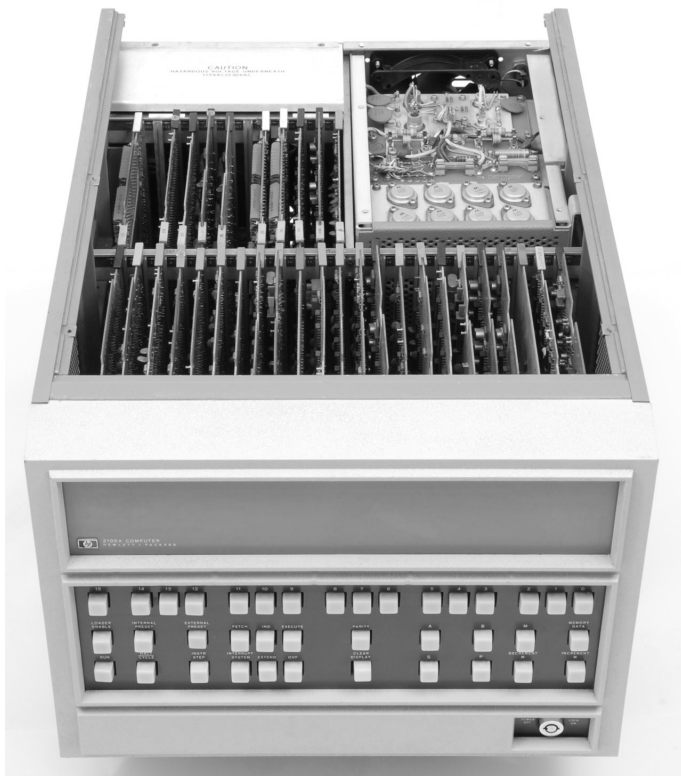
Figure 1.1: The main unit of the HP 2100A mini computer. (Photo courtesy of hpmemory.org, Marc Mislange.)
